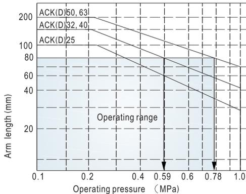
Example: When arm length is 80mm, pressure should be less than
