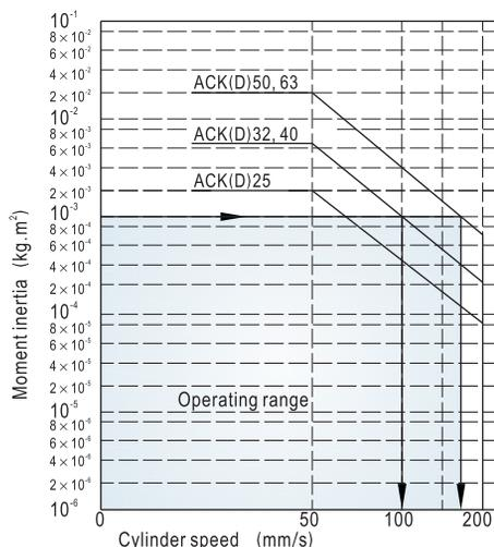
Example: When arm's moment of inertia is  $10^{-3} \text{Kg} \cdot \text{m}^2$ , cylinder speed should be less than
