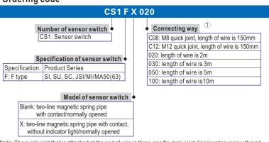
① Note: The quick joint that is attached at the end of wire is three-needle-male joint-linear-rotary screw thread type. The female joint plug has to be ordered additionally. Please refer to P442 for the specific data.
